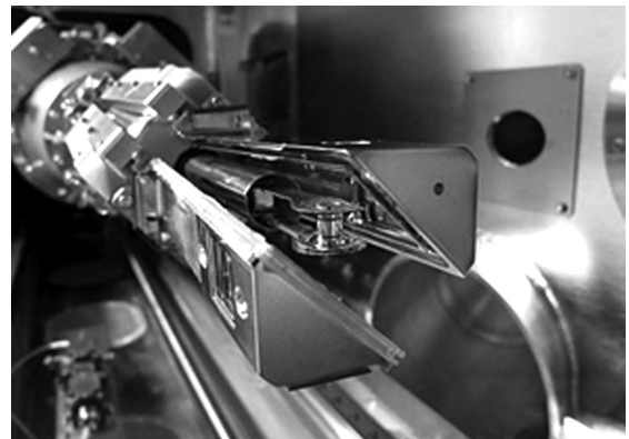
Figure 3: The target assembly for NIF's first integrated ignition experiment is mounted in the cryogenic target positioning system
